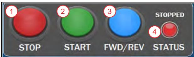
1. **STOP button:** stops the pump from running.
