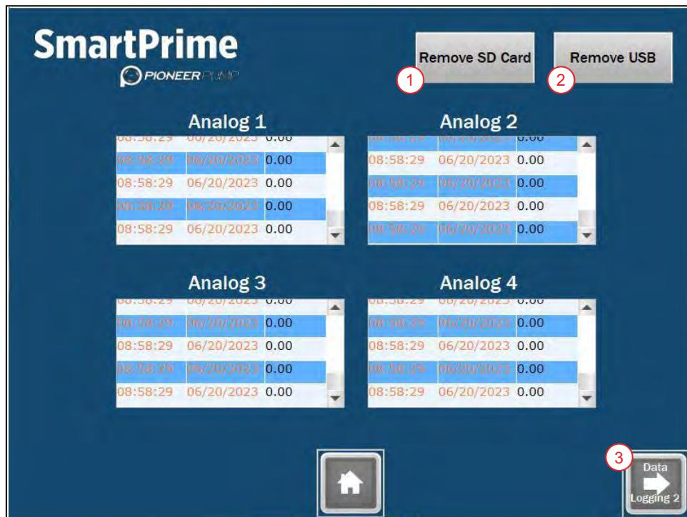
1. Remove SD Card button: press before removing the SD card from the HMI to discontinue writing.
