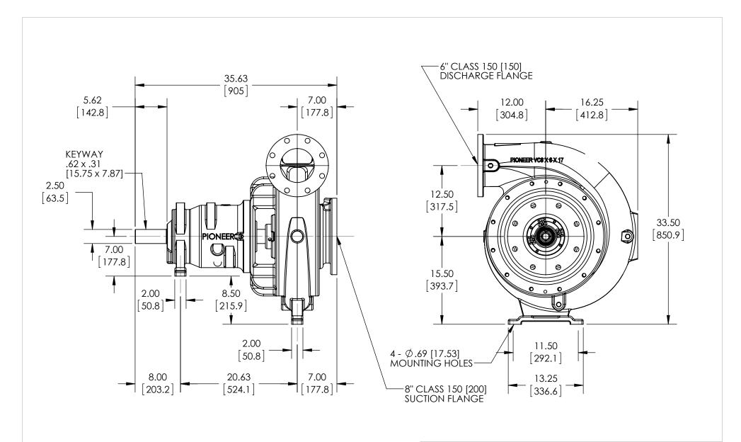
DIMENSIONS ARE IN INCHES AND [MILLIMETERES]. UNLESS OTHERWISE SPECIFIED, TOLERANCES ARE ±0.125 [3.2]
