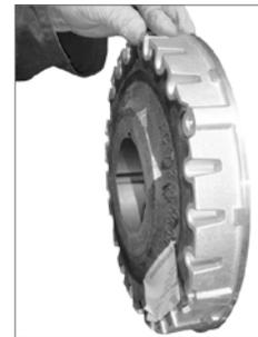
To be conservative, it is good to have the edge of the metal spline protruding as much as 1/8" (3 mm) beyond the rubber spline and not less than flush between the two parts. On the pump, the fit between the drive shaft key and its keyway should be checked for proper fit. If they are too tight, use a file to adjust to a snug fit between the two parts.
