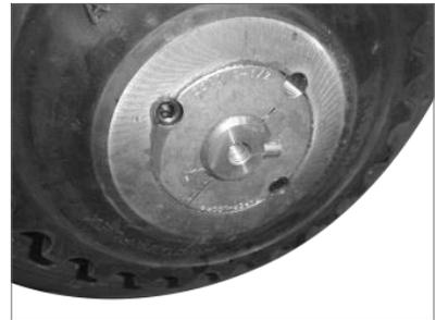
7. Apply Loctite<sup>®</sup> 243 or similar to the set screws and install them in the hub, ensuring that the correct two holes are used. The third hole is threaded and is used as a "jacking hole" during disassembly. The set screws should be tightened to 175 ft-lbs (237 Nm).
