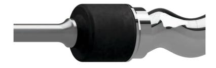
Fully Sealed Universal Joint: where neither ingress of chemical product nor contamination of the product by the lubricant within the joint can be tolerated. The fully sealed universal joint provides complete sealing protection. Typical applications are food products and explosive slurries
